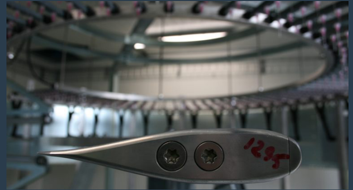
A sample of Doncasters Bramah's metal alloy undergoes testing at the Catapult's Rain Erosion Test Rig in Blyth.
