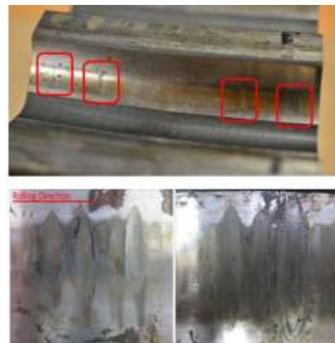
Figure 2- Examples of worn pitch bearing.
