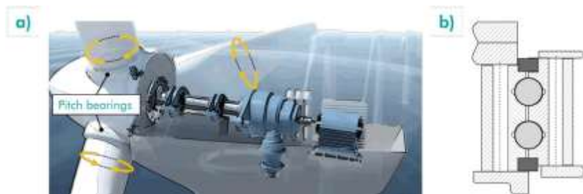
Figure 1- a) Pitch bearing (image: schaeffler-fairs.de) b) Typical double-rowed four-point contact ball pitch bearing.
